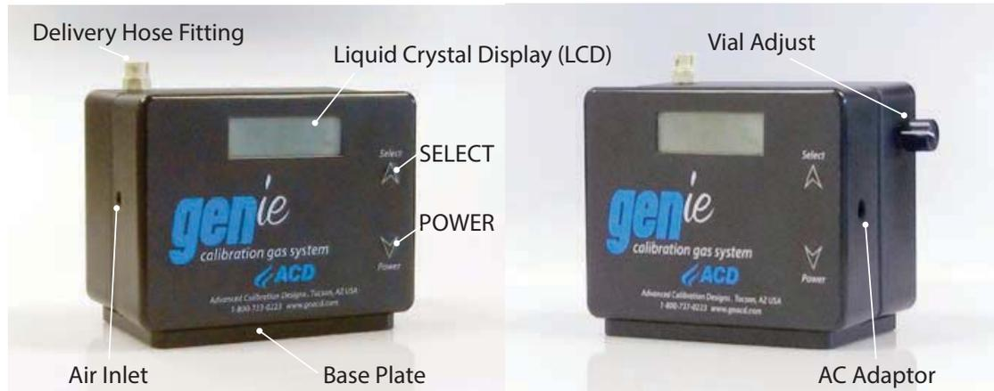
The GENie base unit has a liquid crystal display (LCD) located on the front of the instrument. This display is protected by a thin, clear plastic cover that is part of the front membrane panel and may be replaced if it becomes scratched or unclear.
