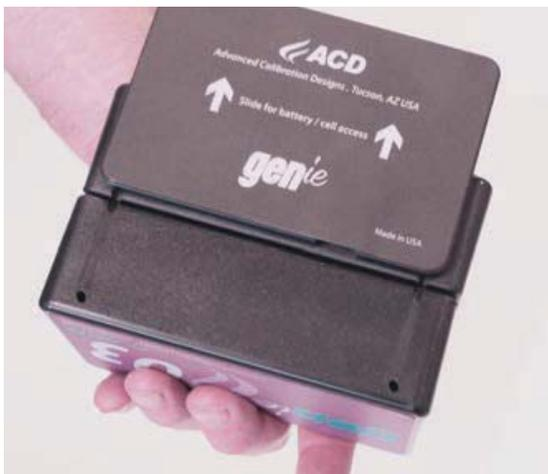
The source module is now disengaged from the base module and can be pulled away revealing the battery compartment.
