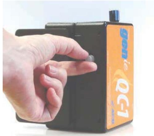
To start the instrument, press and hold the POWER switch, located in the lower right of the front of the instrument, until the display reads **GENie QC-1**, approximately five (5) seconds. Release the switch immediately thereafter.
