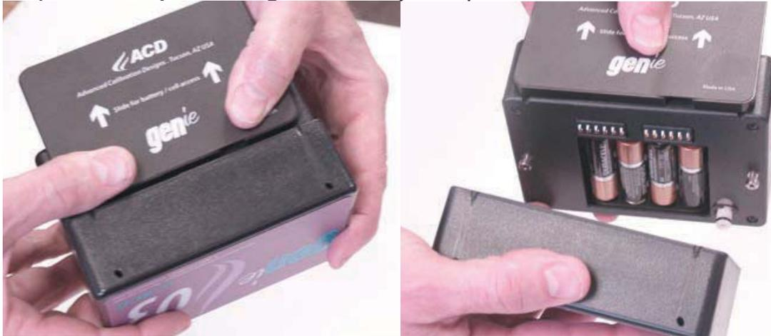
To reinstall the source module onto the base module, take the following steps: Align the air inlet fitting and the locking pins into the eyelet holes as shown. Press the two units together and slide the source module upwards (relative to the base module) to lock it in place. The two units should be flush and tightly secured at this point, then simply slide the base plate back into position until it latches.
