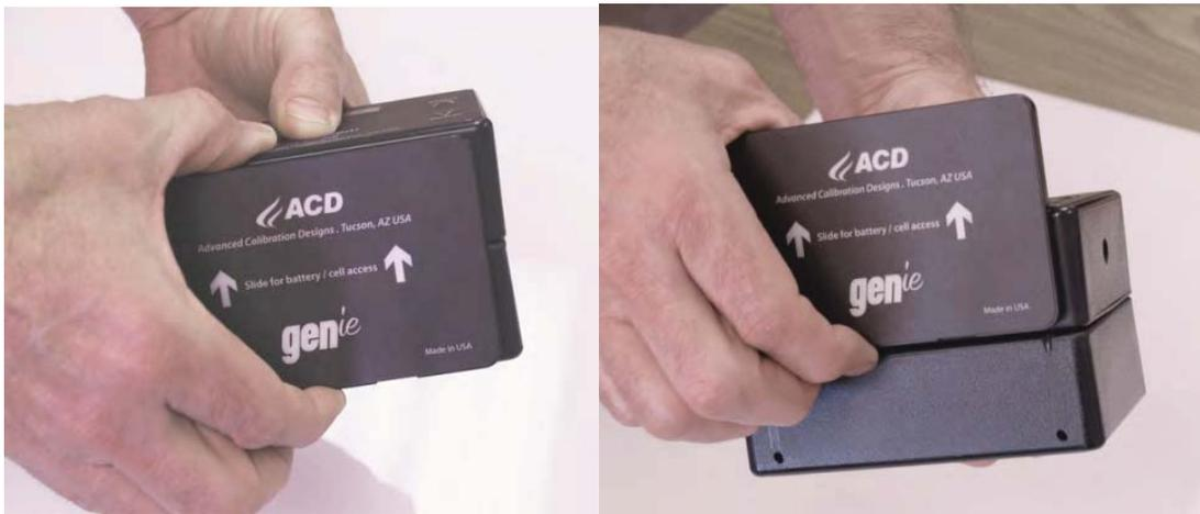
With the base plate out of the way it is now possible to disengage the source module. This is accomplished by sliding the source module downward (relative to the base unit) as shown.
