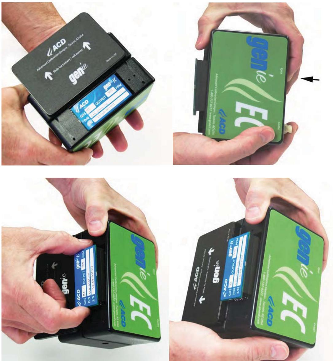
Install the new cell by aligning the cell contacts and pressing the cell in until it stops. Slide the base plate in the opposite direction of the arrows until it snaps in place.
