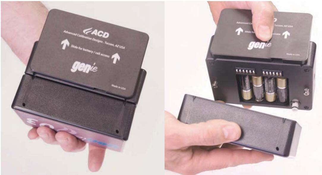
To reinstall the source module onto the base module, take the following steps: Align the air inlet fitting and the locking pins into the eyelet holes as shown. Press the two units together and slide the source module upwards (relative to the base module) to lock it in place. The two units should be flush and tightly secured at this point, then simply slide the base plate back into position until it latches.
