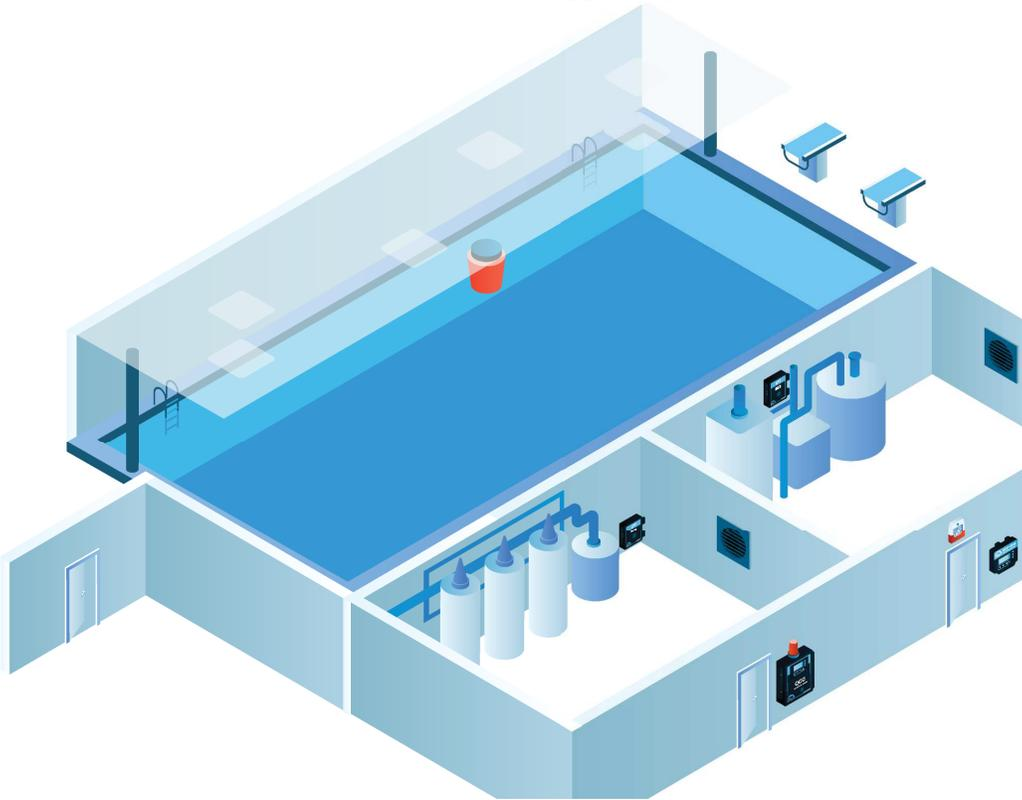
The LPT-A-CL2 remote transmitter should be mounted inside the Chlorine gas feed and storage room, close to the area of a potential leak to provide continuous monitoring. Chlorine is heavier than air and tends to collect in low-lying areas, so the LPT-A-CL2 transmitter should be mounted 6 inches above the floor.
