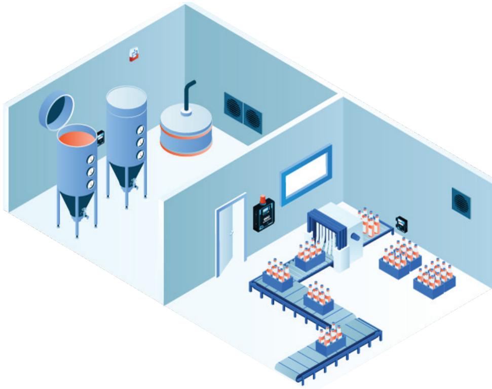
During the bottling process, CO<sub>2</sub> is used to pre-fill each bottle before it is filled with beer. Another CGAS Detector with a CO<sub>2</sub> infrared sensor should be mounted in the bottling area to monitor and protect workers on the bottling line. The cGAS Detector CO<sub>2</sub> transmitter is available with analog output (p/n: CGAS-A-CO2-5%) or Modbus output (p/n:CGAS-D-CO2-5%).
