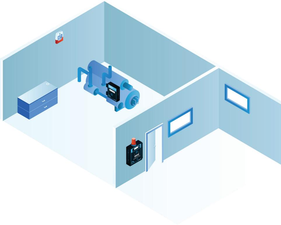
The CGAS-A-IR will continuously transmit a 4 - 20 mA analog signal to the DCC Controller which will show the corresponding gas level readings. The DCC should be mounted at viewing height outside the chiller room door so the display can easily be seen prior to entering the room. There should be a remote visual and audible alarm device inside the room and outside any other entrance door to the room.
