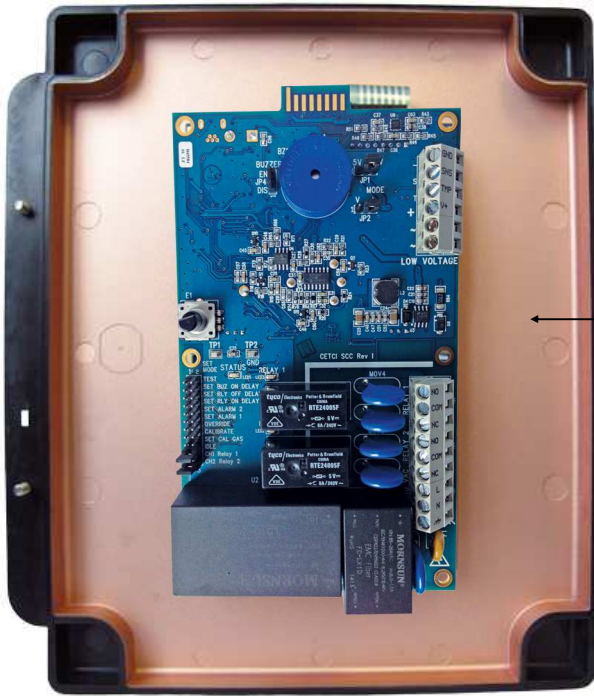
SCC TYPE "A" 1-CHANNEL SELF-CONTAINED GAS DETECTION SYSTEM. ONE INTEGRAL CO OR NO2 SENSOR
