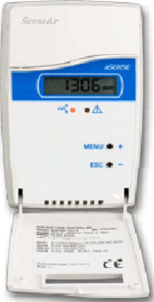
Figure-11 The ENTER command is done by pushing buttons MENU and ESC at the same time for about 14-seconds
