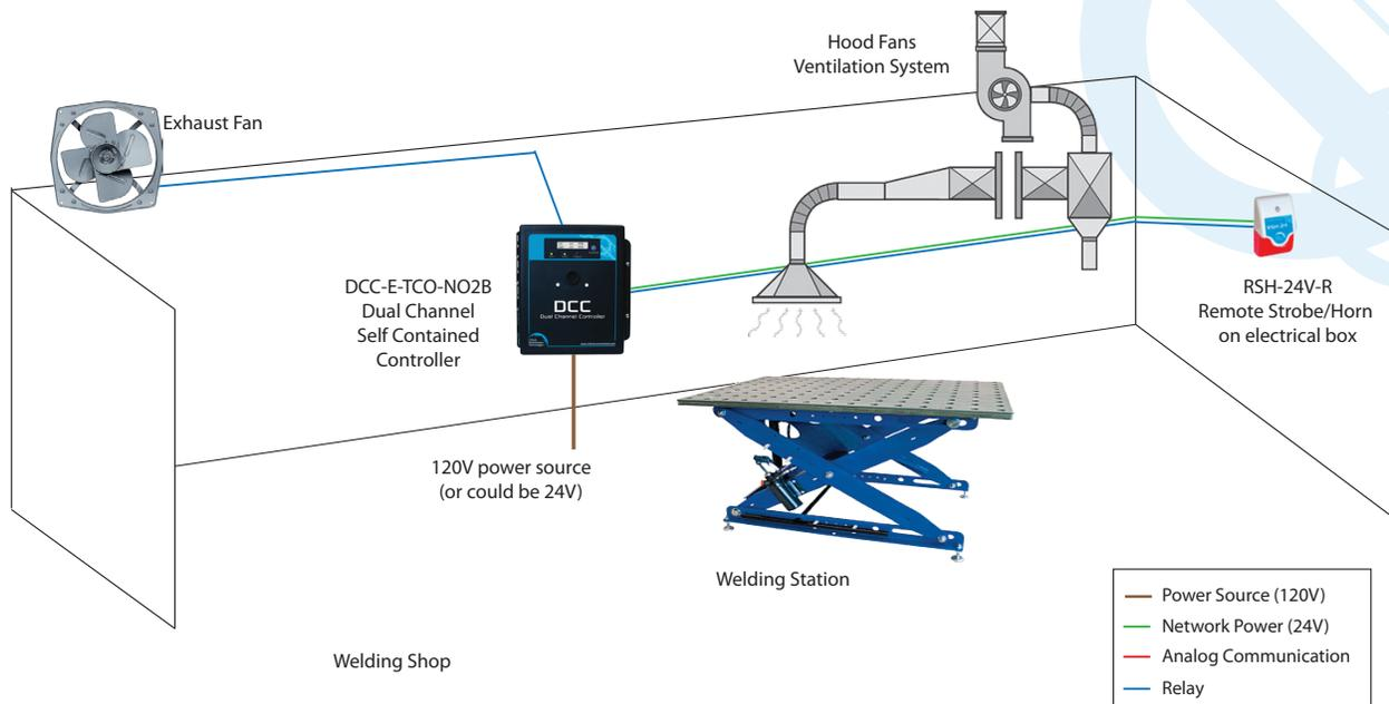
Welding activities occur in many industries and the work environments vary in size, layout and setup. When planning installation and mounting locations for each DCC Dual Channel Controller, you must consider the air flow patterns in the room. Entrances to the room, type of ventilation system, number of welding areas and any other sources of active air currents will affect the ability of the sensors to accurately read the gas levels.
